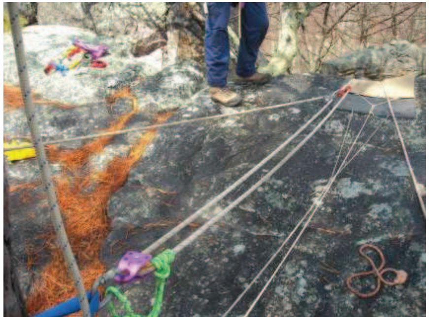
A 3-1 (Z-rig) with a PMP & prussik PCD. (Prussik- Minding Pulley with a prussik Progress Capture Device.)The line at the right is the Belay line.
